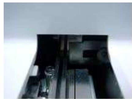
After the size of the screws are set, adjust the stop piece of the feed bin via the panel, otherwise the screw will come out from the feed bin.
