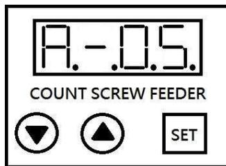
Screw feeding speed setting: Press ▲▼ to adjust:
