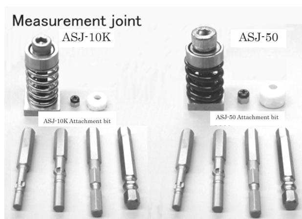
The bolt omission prevention function was newly carried in joint. By attaching an omission prevention screw, if a bolt separates from a plinth, it will race, and it does not decompose and trouble is not caused to work. (However, when it continues racing, a ridge may be worn out and torque value may change.) Moreover, by wear, the metal fatigue, etc. of a screw, where a spring is closed, it is left, and a bolt may jump out with the pressure.
