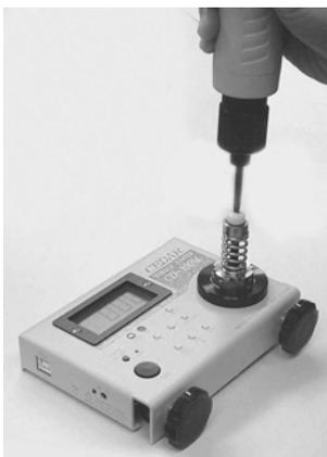
4. The fit of the bit of an electric driver is carried out to the screw of ASJ joint head, operate an electric driver, fasten, and perform lump operation. **It checks whether the spring of ASJ joint is loosening at this time.** When you are not loosening, please be sure to start measurement after loosening.
